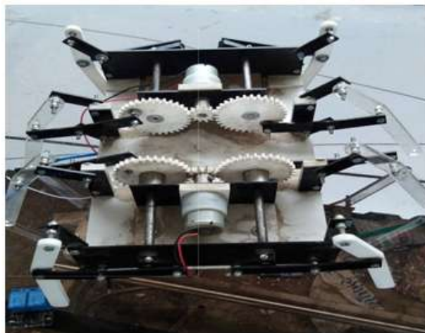
Fig -4: Actual Design Model of Klann Mechanism
